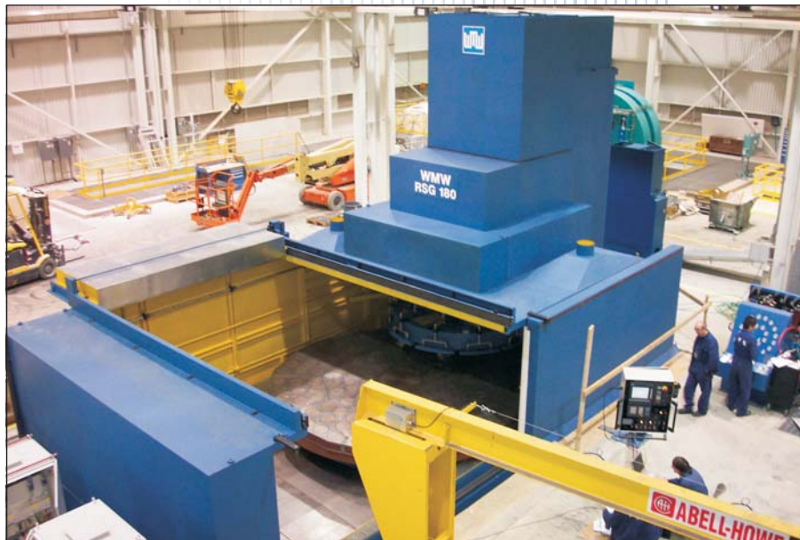
RSG 4570 vertical rotary surface grinder
